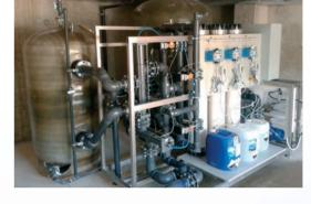
Control panel with microprocessor-controlled PLC system for automatic management, an user friendly touch screen display showing operating parameters as pressure, flow rate, time filtration and backwash, position of each valves, alarm for faults, history...;
